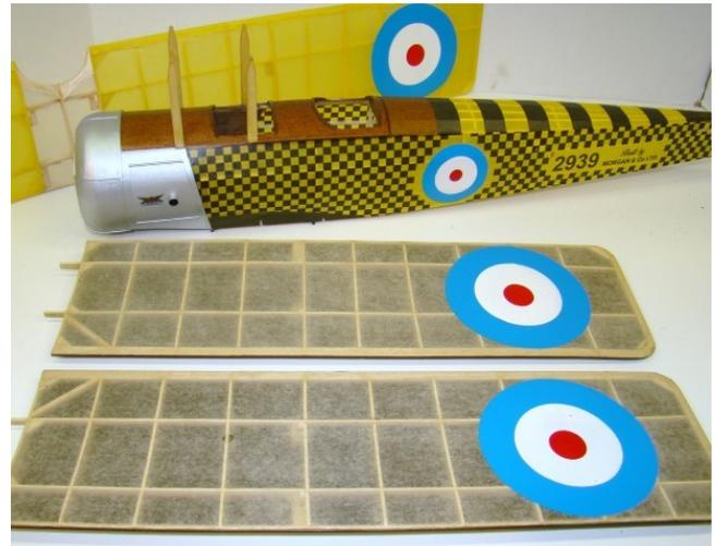
I don't think there is anything left to do but put it all together. In order to add the wings, I first pinned down the fuselage to the building board. The lower wing trailing edges hang below the bottom longerons, so a small platform was made to raise the fuselage up a tad off the building board. After what seemed like a dozen or so dry runs, the wings were glued on, propping up the wing tips with balsa to give me the desired one inch dihedral plus the height of the fuselage platform.
