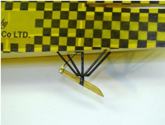
The tailskid and its mount were composed of bamboo and basswood. A small piece of brass sheet was wrapped around the end of the tailskid, and copper wire was added to mimic the cable that travels up inside the fuselage that I presume attaches to a shock cord.
